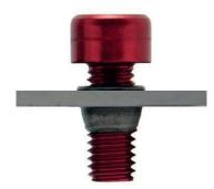
Formdrills use rotational speed and axial force to produce friction. This friction heats up the material and softens it enough to make a hole and displace the material to form an insert.
